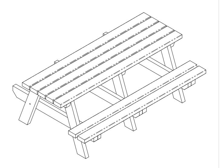
3. To finish the assembly tighten all bolts. Fit nut covers on the table top mounting bolts.
