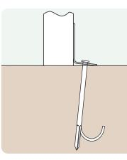
Anchored Soft ground fixing kit for grass.
