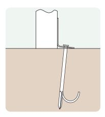
Anchored Soft ground fixing kit for grass.
