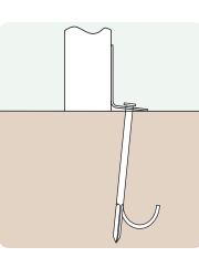
Anchored Soft ground fixing kit for grass.
